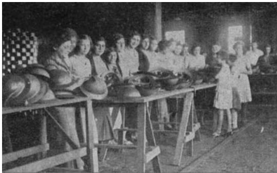
Women assembling liners and chinstraps on the British model Mk I in 1932. Stamped helmets, lacking the painting, the liner and the chinstrap (newspaper's section-Author's collection)
